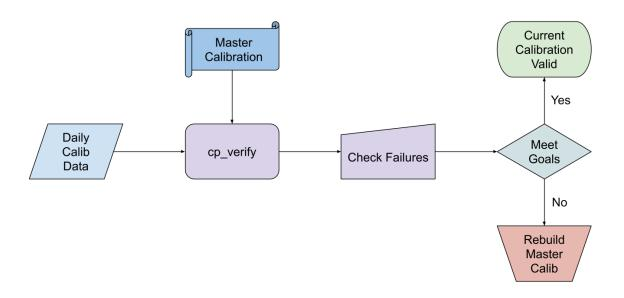
FIGURE 2: Flowchart of the daily calibration process.
